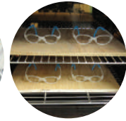
Temperature stability test
